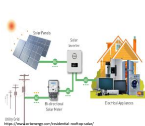
Grid-connected rooftop solar systems
